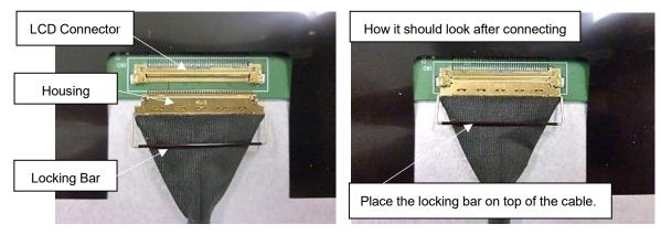
(2) Fit the Locking bar into the LCD Connector (Locked)
