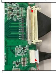
Insert with the connecting point facing up not visible.
