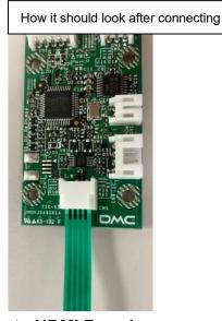
9-4 Connecting Image Cable to HDMI Board
