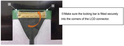
(3) Secure the locking bar with insulating tape so it will not come off (not required but recommended).
