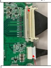
Insert with the connecting point facing up not visible.
