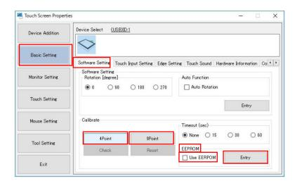
(3) Click and place a check in the box next to [Use] under [EEPROM] and click [Register]. When [4 Point Correction] or [9 Point Correction] is performed with the check in the box, the correction data will be stored in the EEPROM of the Product.
