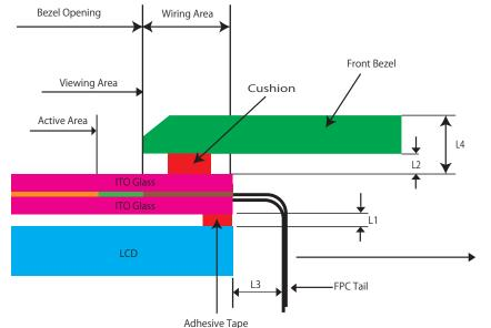
L4≧2mm: Distance between touch screen and bezel surface
